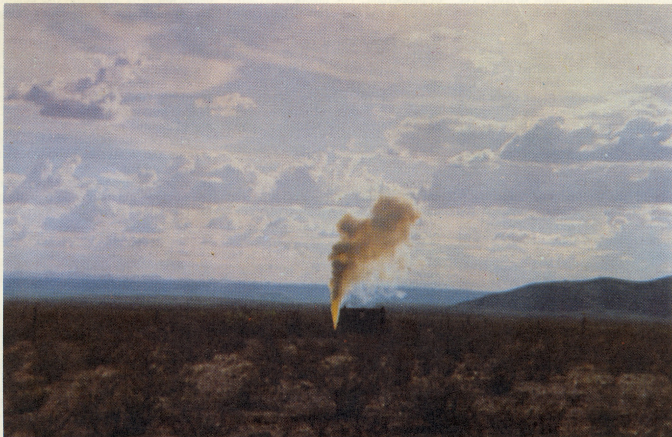
FIGURE 2. Static test firing of the motor. The flame is approximately 7 ft. long.
