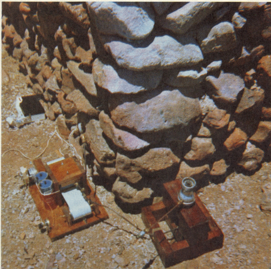
FIGURE 1. Moving clockwise the photo shows the tape recorder, graph recorder, and rocket motor. A similar but larger motor was used in the test described in this paper.
